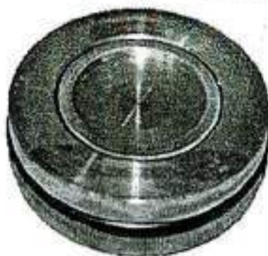
Figure 4: Silicon Cut Silicon Single Crystal Zero Background holder with Kapton film
