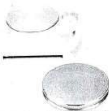
Figure 1: Pictorial Presentation of Backloading Holder (Courtesy: Malvern-Panalytical X-ray diffraction manual and X'Press magazine)
